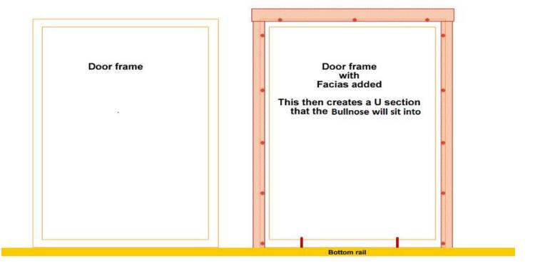
Now we need to add the Bull nose uprights into the hole in the wall, these uprights must not be screwed/fixed in any direct way to any of the log cabin logs as standard ... However again some fitters will send a screw through the bullnose into the very bottom logs of the cabin ONLY for support.
